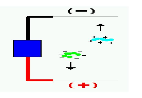
**Electrophoresis** is a technique used for sorting of macromolecules molecules <u>based on size</u> <u>and charge</u>.
