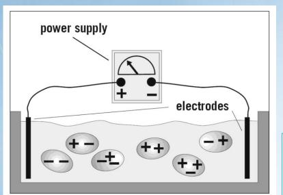
Proteins move in the electric field. Their relative speed depends on the charge, size, and shape of the protein
