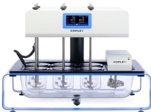
The most common apparatus used to measure the dissolution rate of solid dose forms are the basket and paddle.
