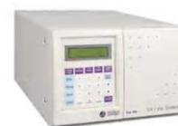
2. **Fluorescence Detector:** wave length rang (220-700nm) for excitation and emission wave lengths.
