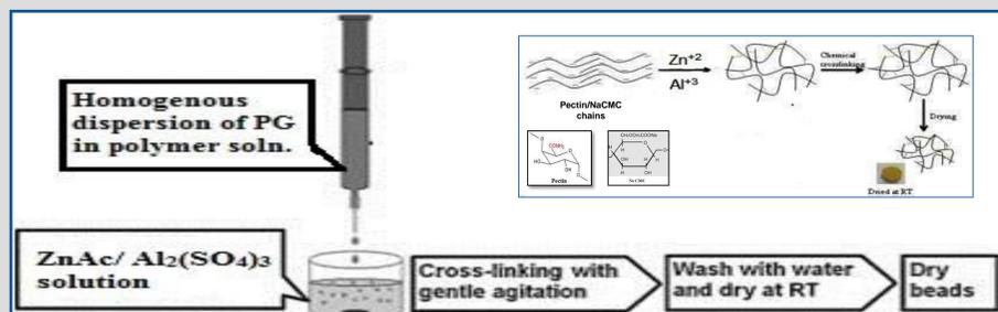
Figure(2) The ionotropic gelation method
