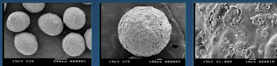
Figure(5) Surface morphology of drug-loaded pectin/NaCMC gel microparticles as appears under SEM
