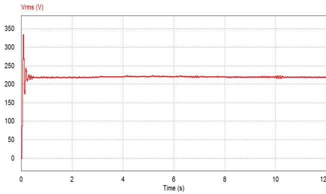
Figure 10. Rms output voltage with  $K_p=0.0001$ ,  $K_i=0.001$  For inductive loads
