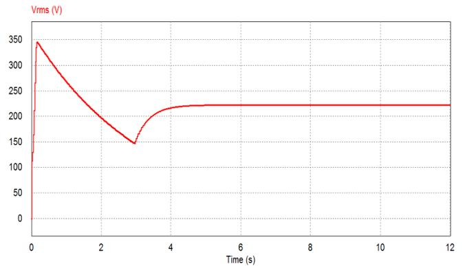
Figure 20. Rms output voltage with  $k_p=1$ ,  $k_i=0.4$  For inductive loads.
