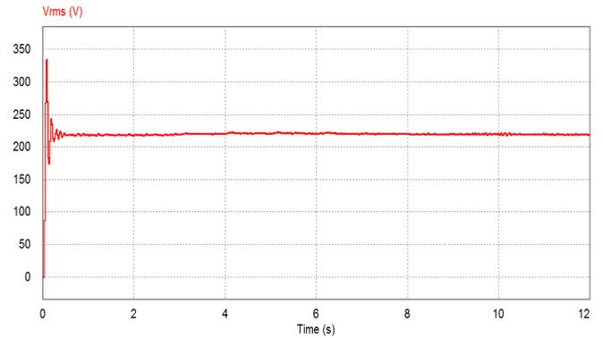
Figure 8. Rms output voltage with  $K_p=0.0001$ ,  $K_i=0.001$  For resistive loads.
