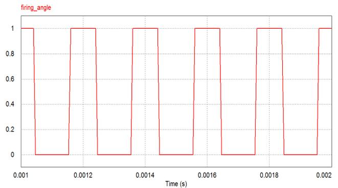
Figure 15. Firing angle of inverter with time for inductive loads.
