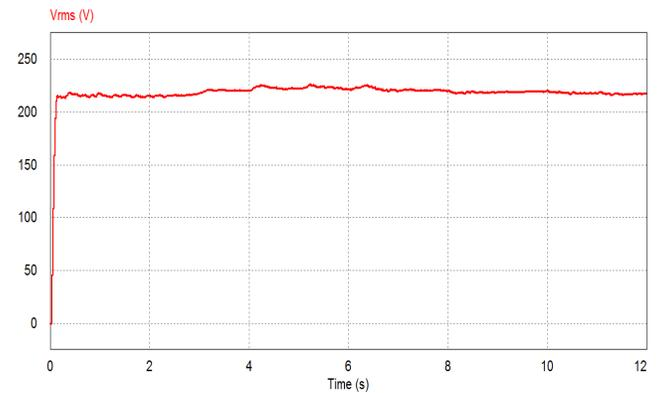
Figure 9. Rms output voltage with  $K_p=0.0001$ ,  $K_i=0.003$  For inductive loads.
