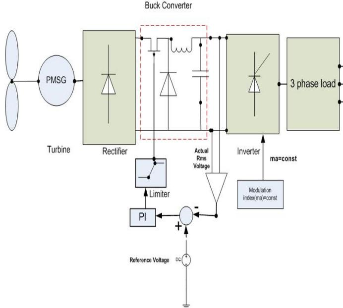
Figure 3. Modified modeling using a switch mode buck rectifier.
