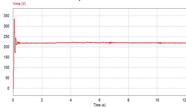
Figure 12. Rms output voltage with  $K_p=0.0001$ ,  $K_i=0.001$  For capacitive loads.
