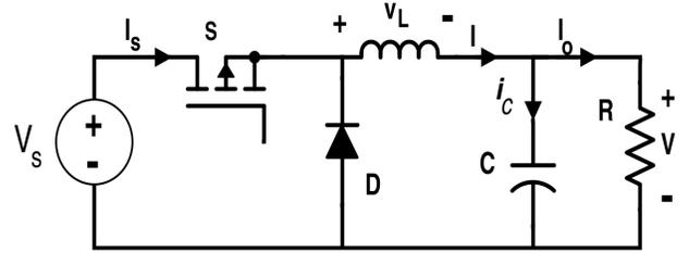
Figure 4. Equivalent circuit of buck converter.
