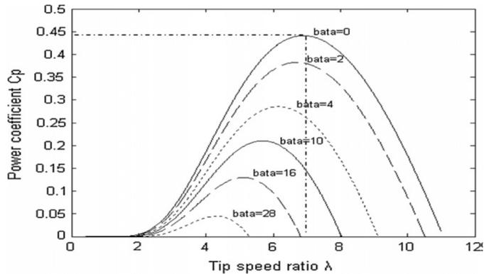
Figure 2. Power coefficient versus tip speed ratio.
