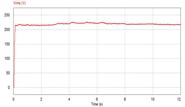
Figure 7. Rms output voltage with  $K_p=0.0001$ ,  $K_i=0.003$  For resistive loads.
