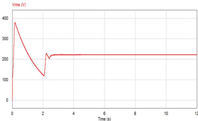
Figure 18. Rms output voltage with  $k_p=1$ ,  $k_i=0.1$  For resistive loads.
