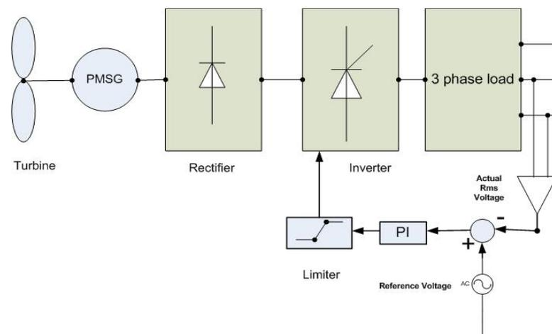
Figure 1. Modeling of the system using voltage source inverter.
