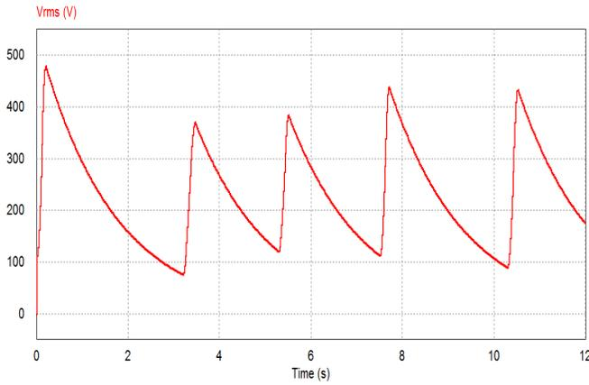
Figure 22. Rms output voltage with  $K_p=1$ ,  $K_i=0.008$  For resistive loads.
