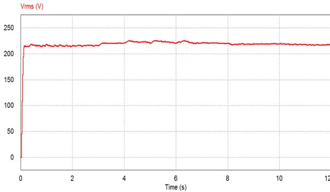
Figure 11. Rms output voltage with  $K_p=0.0001$ ,  $K_i=0.003$  For capacitive loads.
