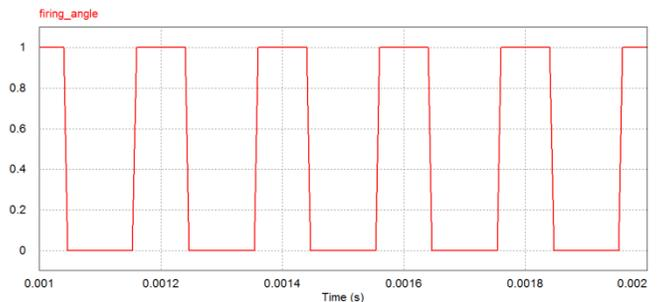
Figure 16. Firing angle of inverter with time for capacitive loads.
