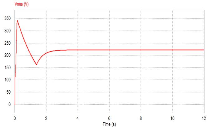
Figure 19. Rms output voltage with  $k_p=1$ ,  $k_i=0.4$  For resistive loads.
