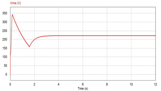
Figure 21. Rms output voltage with  $k_p=1$ ,  $k_i=0.4$  For capacitive loads.
