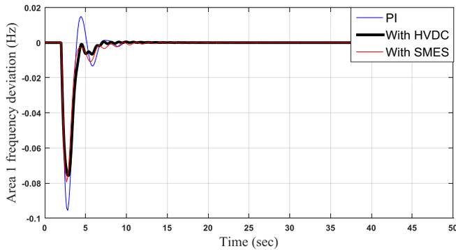
Figure 10. Frequency deviation response of area-1 due to 10% load disturbance at thermal area-1.
