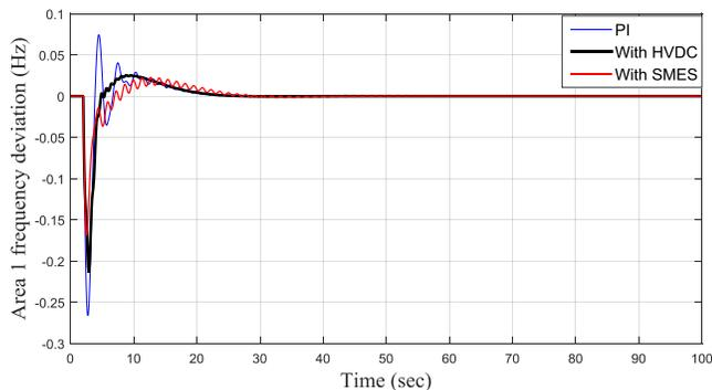
Figure 14. Frequency deviation response of hydraulic area-1 due to 10% load disturbance at hydraulic area-1.
