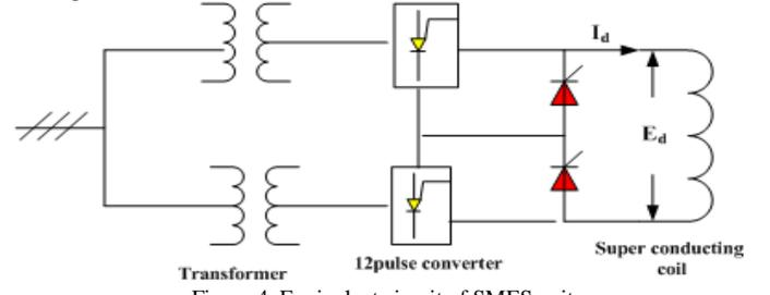
Figure 4. Equivalent circuit of SMES unit.
