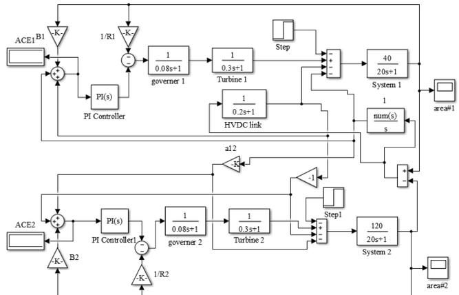
Figure 8. Matlab Simulink model of the proposed HVDC link between two areas interconnected power systems.
