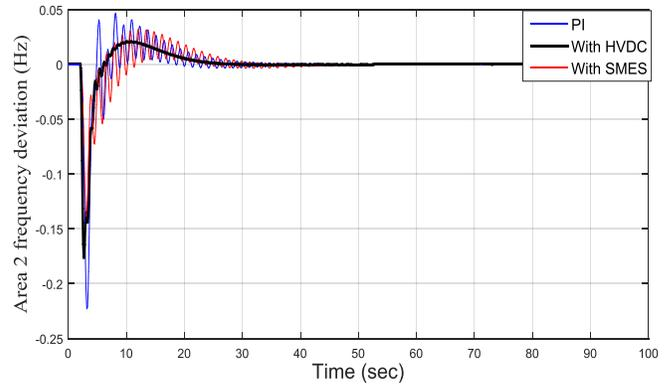
Figure 15. Frequency deviation response of thermal area-2 due to 10% load disturbance at hydraulic area-1
