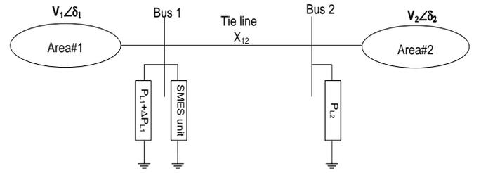
Figure 5. Single line diagram of the two-area power system with SMES unit.
