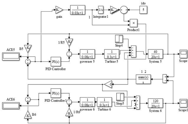
Figure 9. Matlab Simulink model of the proposed SMES systems connected at area-1 of two areas interconnected power systems.
