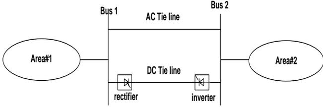
Figure 3. Two areas with AC-DC Tie-Line Connection.
