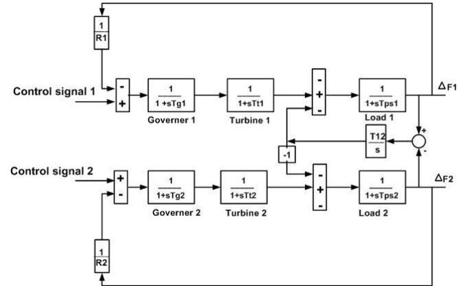
Figure 2. Block diagram of LFC of thermal two area interconnected power system.
