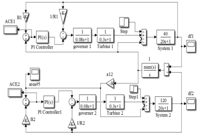
Figure 7. Matlab Simulink model of two areas interconnected power system with two thermal units.
