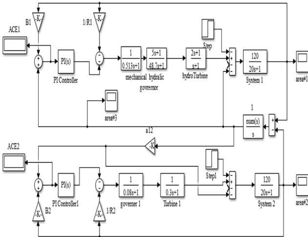
Figure 13. Matlab Simulink model of two areas interconnected power system with two hydraulic-thermal units.
