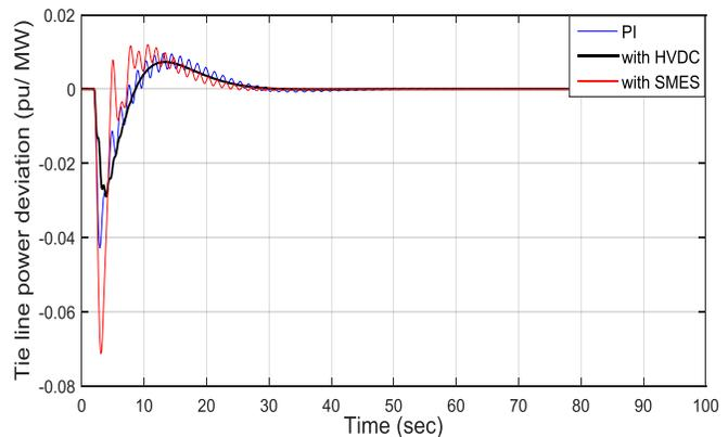
Figure 16. AC Tie line power deviation response due to 10% load disturbance at hydraulic area-1.
