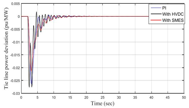
Figure 12.AC Tie line power deviation response due to 10% load disturbance at thermal area-1.
