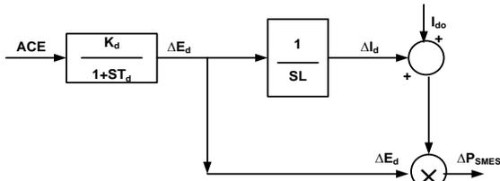
Figure 6. Block diagram of SMES unit control system.
