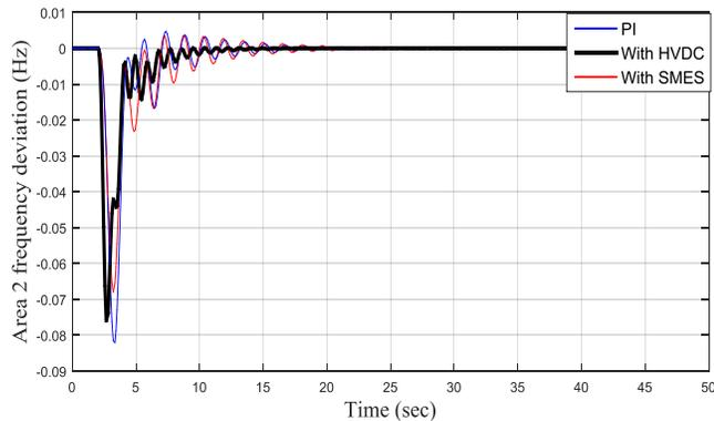
Figure 11. Frequency deviation response of area-2 due to 10% load disturbance at thermal area-1.
