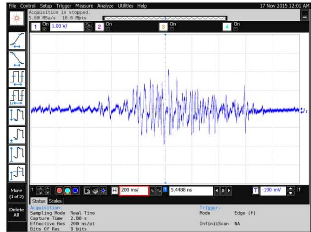
Fig. 3. EMG signal sensed from the biceps muscle displayed by Agilent Digital Oscilloscope
