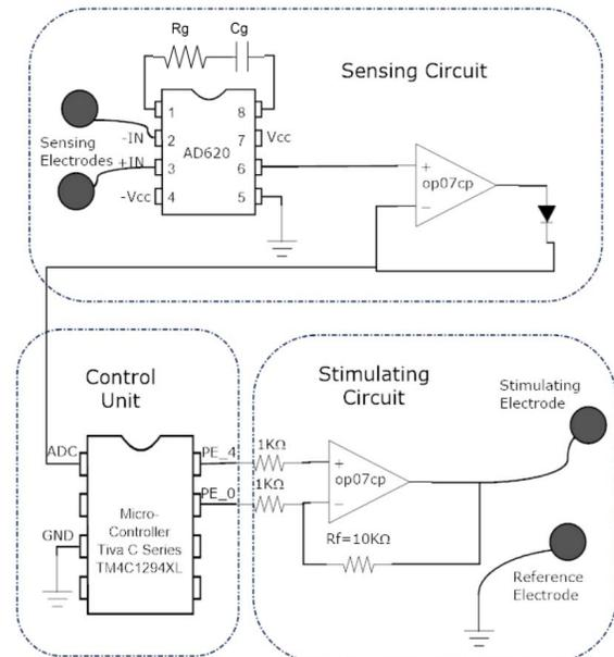
Fig. 1. Schematic diagram for the system of sensing and stimulating EMG signal in muscles
