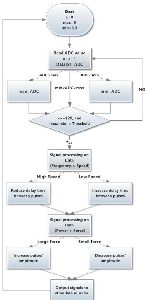
Fig. 6. Flow chart showing the process flow in the microcontroller
