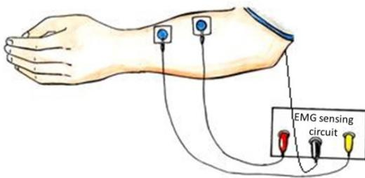
Fig. 2. Placing EMG sensing electrodes on the muscle
