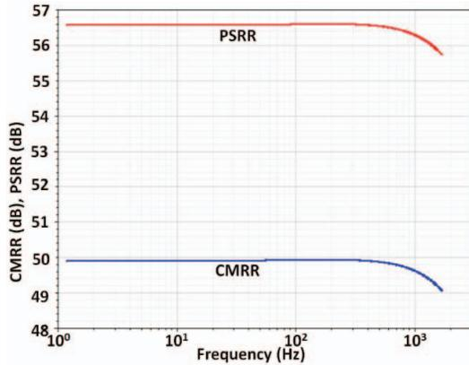
Fig. 6. CMRR and PSRR of the proposed design.
