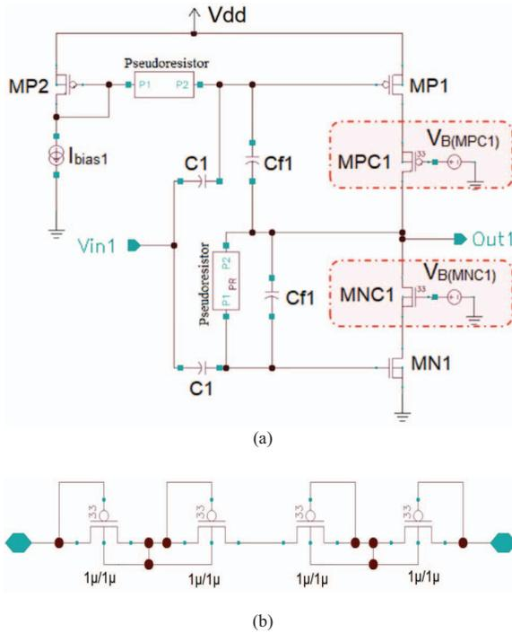
Fig. 2. (a) Schematic of the first-stage amplifier. (b) Pseudoresistors used in first and second stages.
