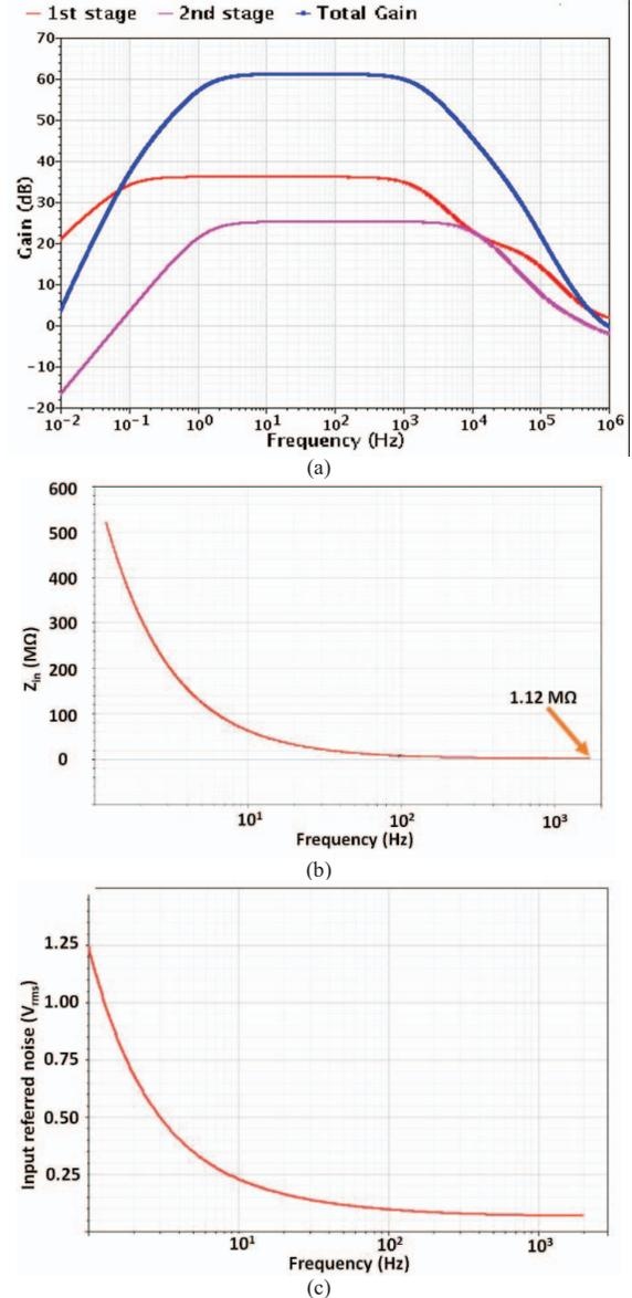
Fig. 5. (a) Frequency response of the first stage, second stage and full amplifier. (b) The input impedance ( $Z_{in}$ ). (c) Input-referred noise spectrum of the proposed amplifier.
