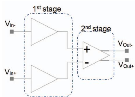
Fig. 1. EMG signal amplifier configuration
