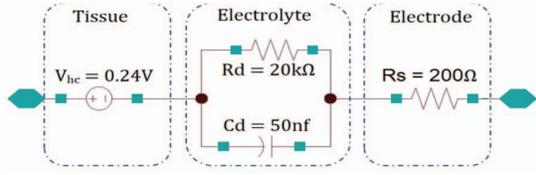
Fig. 4. Equivalent circuit for biopotential electrode.
