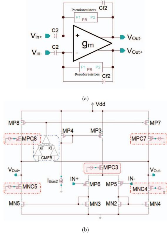
Fig. 3. (a) Schematic of the second-stage amplifier. (b) Schematic of the OTA.
