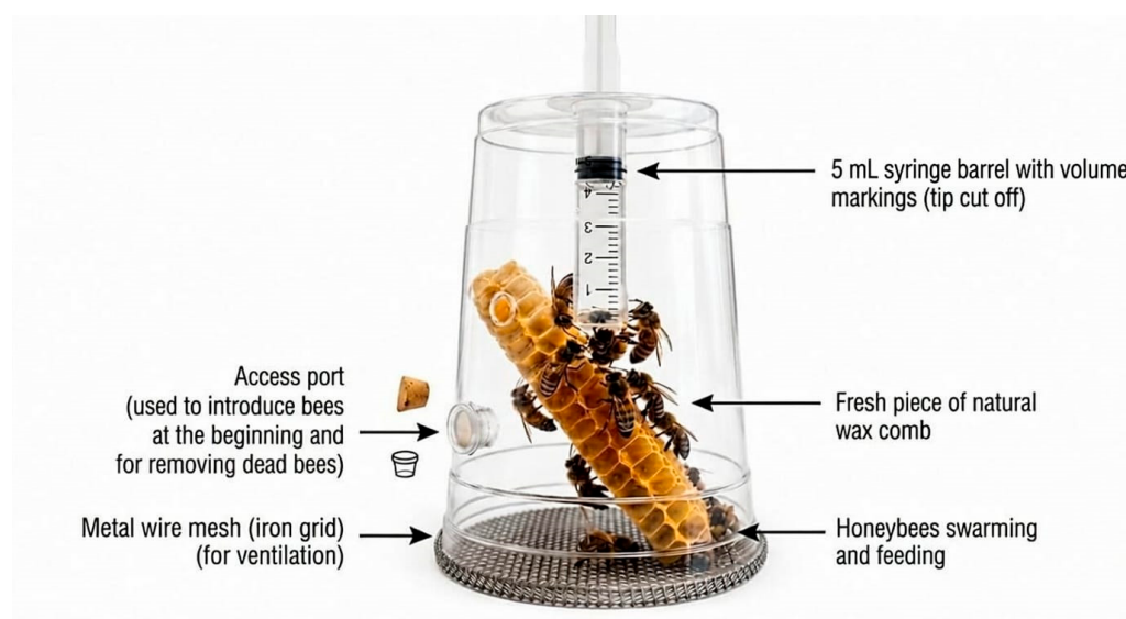
Figure 1. Plastic experimental cage used for oral toxicity bioassays on adult honeybee workers under laboratory conditions.
