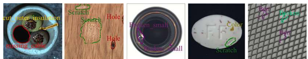
Fig. 1. Some cases show multiple, varied defects.
