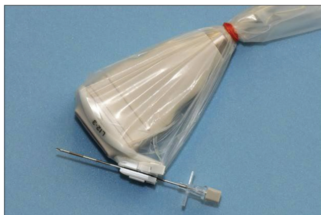
Figure 1: The needle guide mounted to the ultrasound probe
