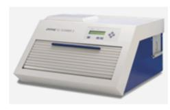
The scanner transmits all measurement data in digital form to the computer for further processing, and features three light sources - a deuterium lamp, a halogen-tungsten lamp and a high pressure mercury lamp which can measure reflection, either in absorbance or fluorescence mode and it has spectral range from 190 to 800 nm with scanning speed 1-100 mm/s and Object formats up to 200 x 200 mm.
