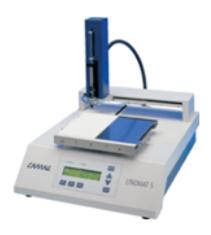
The TLC Scanner 3 is the most advanced workstation for densitometric evaluation of Thin-Layer Chromatograms. It can also be used for densitometric measurements of other planar objects, such as electrophoresis gels. Only the positioning of the object to be measured is performed manually.
