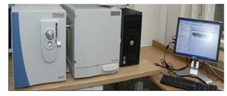
combines the advanced, next-generation curved optics of the industryleading DSQ II with the small footprint of the FOCUS GC to create a compact but powerful analyzer for environmental, petrochemical, forensics, toxicology and QA/QC applications.
