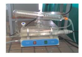
Used for purification of laboratory water
